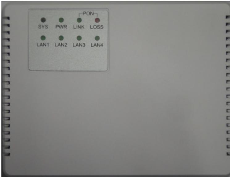
Figure 1-1 Front template of P1004C1
